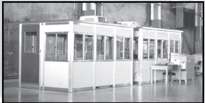
Aircraft maintenance is monitored on hanger floor. Self-contained quality assurance pods are forkliftable and positioned adjacent to tasks.
