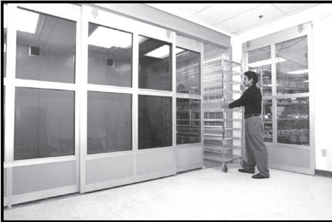
Electronic instrumentation is tested at a constant 131° F prior to acceptance and shipment to the customer.
